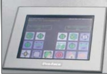
Operator control from 5.7" colour touch panel
