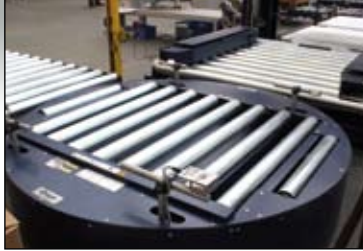
Turntable with integrated roller conveyor
